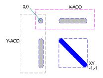
REMEMBER the efficiencies multiply: X-axis = 80%, Y-axis = 80% then XY efficiency = 64%
