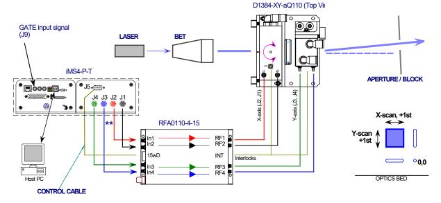
Note: the different connection order between the four iMS4 outputs to the RFA0110-4 inputs.
