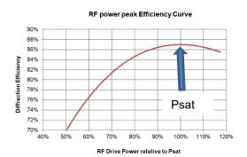
*Tip:* DO NOT overdrive and exceed Psat @ 100%. Better to operate at < 95% and NOT > 100%.
