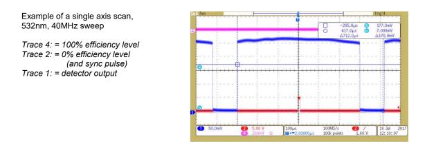
A good LUT will also give a uniform response at lower RF powers e.g. reduce the DDS level to (say) 40%
