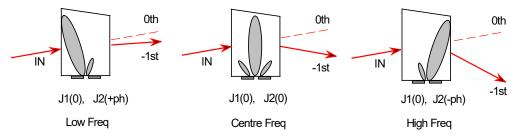
Figure 1: Beam Steering
