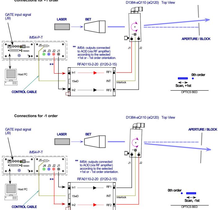
Note: the different connection order between the two iMS4 outputs to the RFA0110-2 inputs.
