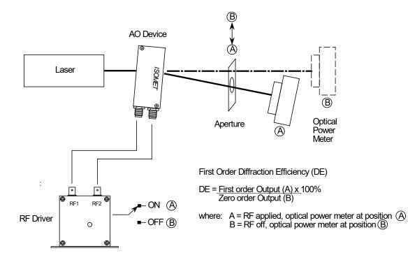
Figure 2: Basic Diffraction Efficiency Measurement
